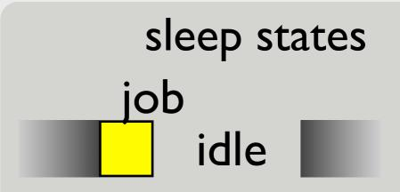
during idle time power consumption is 0, except for the L last units, necessary for wakeup.
